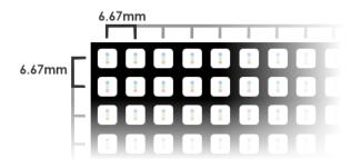
144x432 is the matrix size. This is the number of pixels high (144) and the number of pixels wide (432) of the display. That's **62,208 pixels!** The more pixels, the higher the clarity and amount of detail that can be shown.
